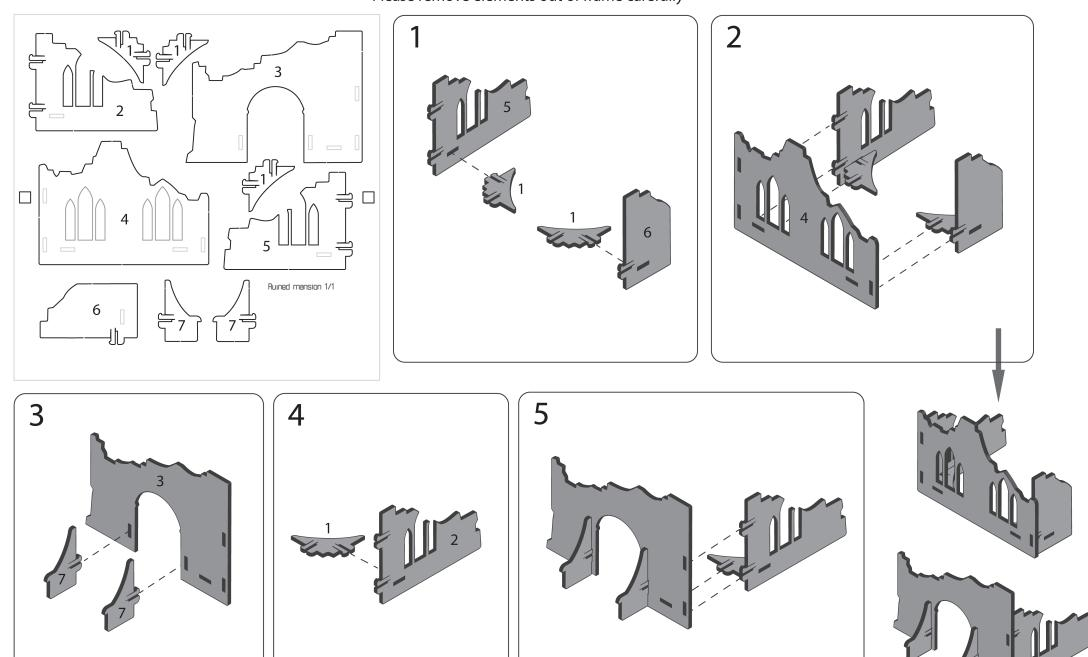
It is recommended to use a blade at the cutline to punch element out of the sheet easier.
